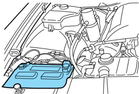
However, for severe usage or in high temperature climates, check the battery electrolyte level. Refer to the “Service Guide” for the service interval schedules.
