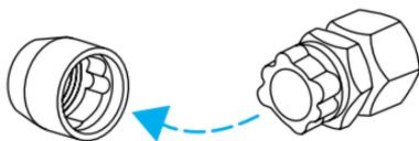
the lug wrench and stored with the spare tire. If you lose the key, send the registration card to the manufacturer (not the dealer) to get a replacement key. If the lug wrench/lug nut key assembly is lost, see your nearest Ford or Lincoln/Mercury dealer who has access to the master set of keys. **Do not use an impact wrench with the anti-theft key.**
